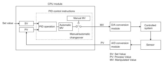
In the PID control processing method, as shown above, the PID operation is executed using the set value (SV) and the process value (PV) read from the A/D converter module, and the manipulated value (MV) is then calculated. The calculated MV (manipulated value) is output to the D/A converter module.
