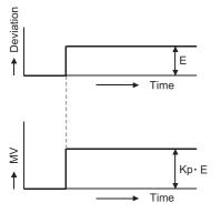
• A certain error produced relative to a set value is called an offset. An offset is produced in proportional operation.
