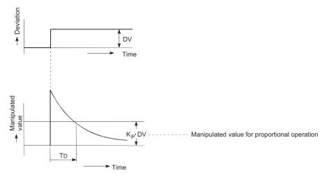
• Derivative operation is always used in combination with proportional operation (PD operation) or with proportional and integral operations (PID operation). Derivative operation cannot be used independently.
