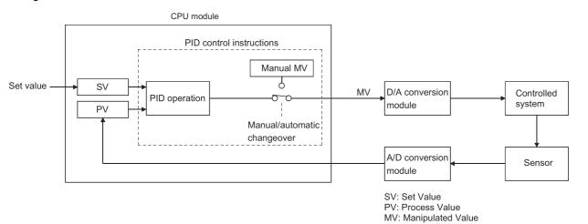
During PID control, the value measured by the sensor (process value) is compared with the preset value (set value). The output value (manipulated value) is then adjusted in order to eliminate the difference between the process value and the set value.
