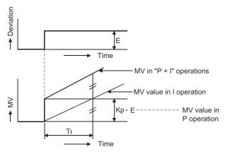
• Integral operation is always used in combination with proportional operation (PI operation) or with proportional and derivative operations (PID operation). Integral operation cannot be used independently.
