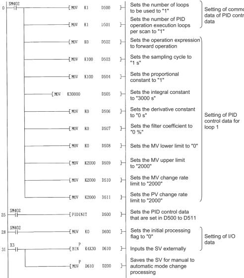
Setting of common data of PID control
