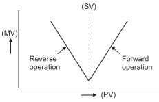
• The figure below shows examples of process control with forward operation and reverse operation:
